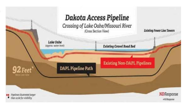
» Figure 3-9. Conceptual site plan for the DAPL's Lake Oahe HDD crossing from draft EA, 2015.
