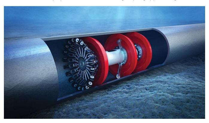
» Figure 5 7. Depiction of a typical smart pig in use in a pipeline.
