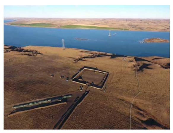
» Figure 5-3. Typical weld string for the DAPL before placement in trench (not HDD).
