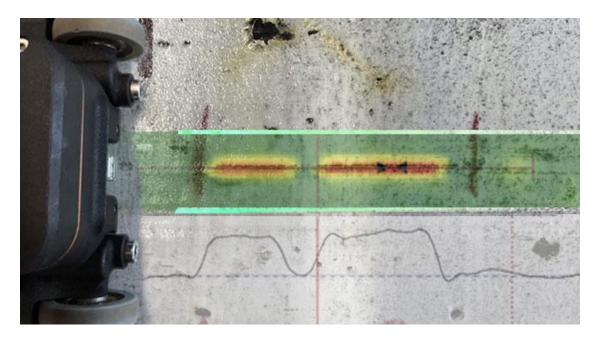
» Figure 5 6. Pinholes of varying stages and diameters in a welded seam.
