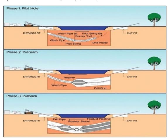
» Figure 5 1. Horizontal directional drilling procedure
